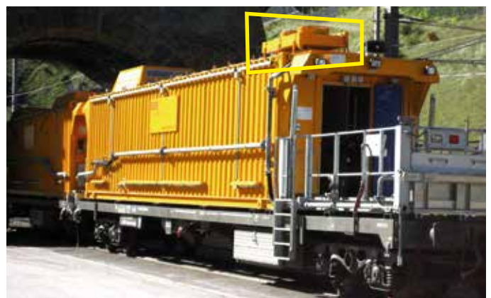
Radiator mounted separately on wagon roof
