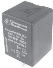
Frequency relays measure the frequency on PIN 15. If the frequency value is bigger than the defined value the relay switches. To avoid wobbling the switch-off threshold is lower than the switch-on threshold.
