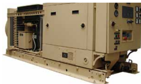
Panda 12 Combo for 12kW electrical power or 12 kW electrical or 7kW + 5kW cooling (24,000 BTU) ECU. Suited for larger power applications using M997 HMMWV ambulance shelter variants.
