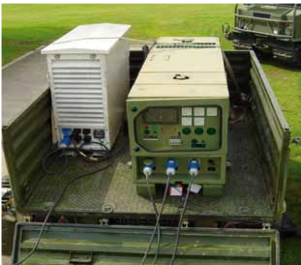
Fully self-contained mounted on frame. The frame base can be transported by fork-lift. The major electrical connections are grouped on the side of the cabinet.
