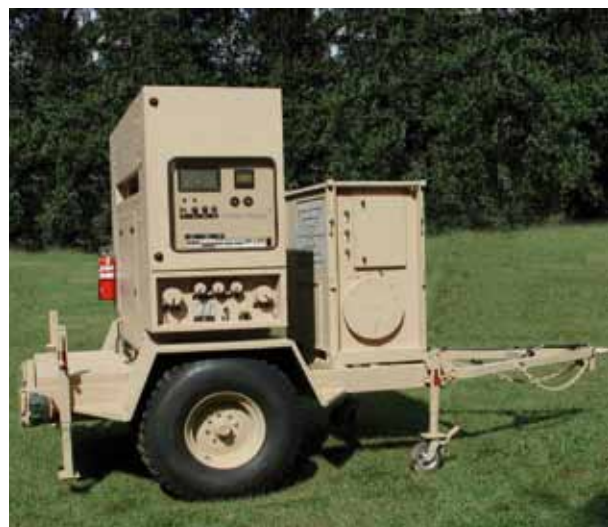
Complete unit, cooling, fuel for 72 hours, 15 kW generator and electrical cabinet mounted on frame. Major electrical functions via remote control unit.
