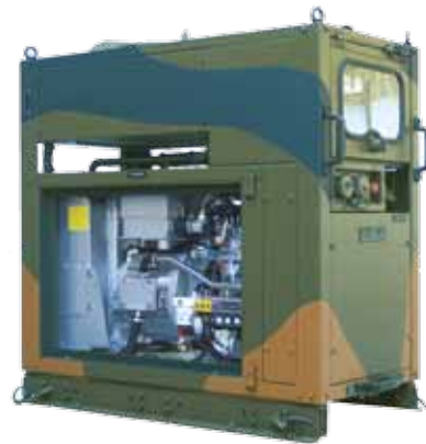
Fully self-contained 8 kW generator with horizontally mounted radiator (tall-version). The unit is mounted on slides which allow 100% extension.
