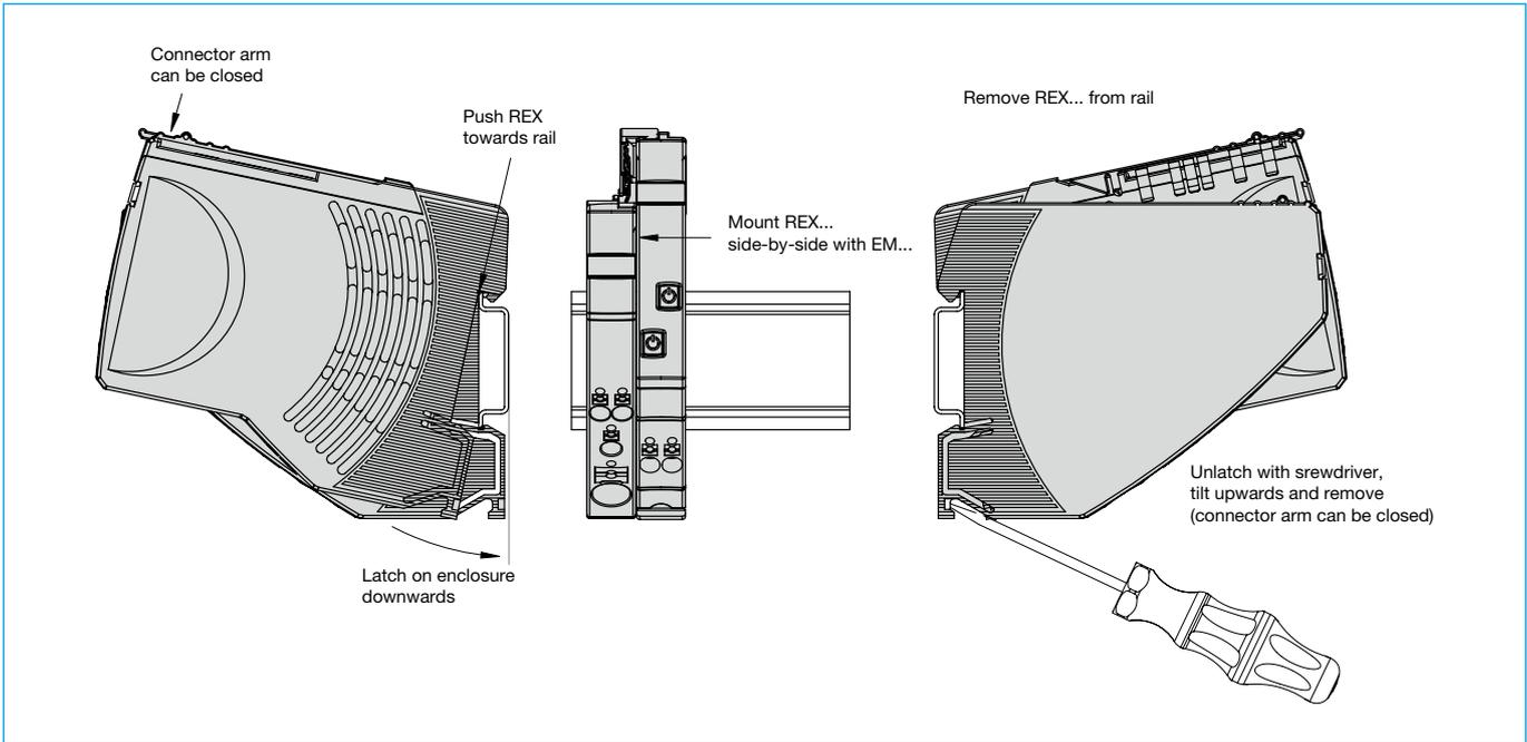
Application example: REX... replacement or disassembly
