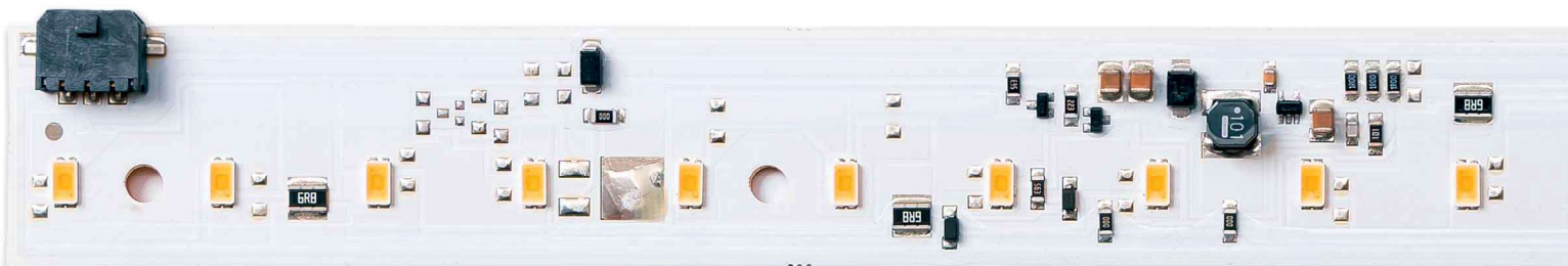
77-146VDC, Constant current, Pulse power supply source, MOLEX connector, OSRAM LEDs DURIS E5, Single BIN Selection
