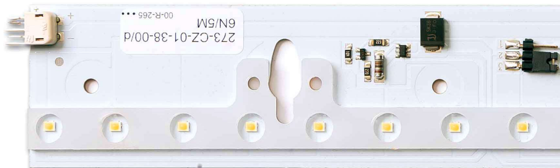
24VDC, Constant current, TYCO connector, OSRAM LEDs DURIS P5, 2BIN selection
