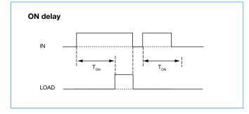
This function allows delayed switch-on of the relay. The configured value indicates the time elapsing between activation and switch-on. Information: Thus the relay may for instance give time to other system components to carry out their start-up, probably attenuating the inrush current peak in the entire system.
