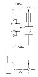
operating condition: 13-14 closed fault condition: 13-14 open
