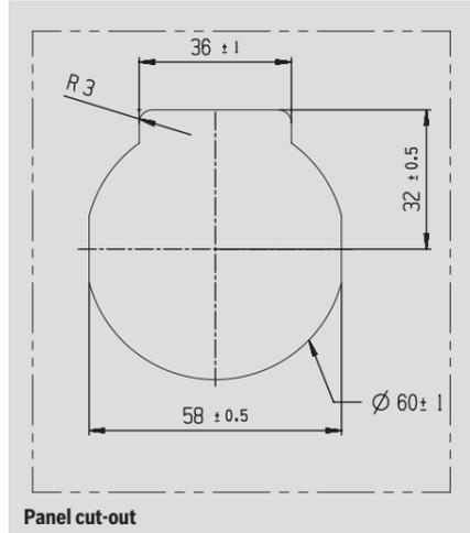
Make sure that there is enough room underneath the panel cut-out for the charging station and its cabling to be dropped in.
